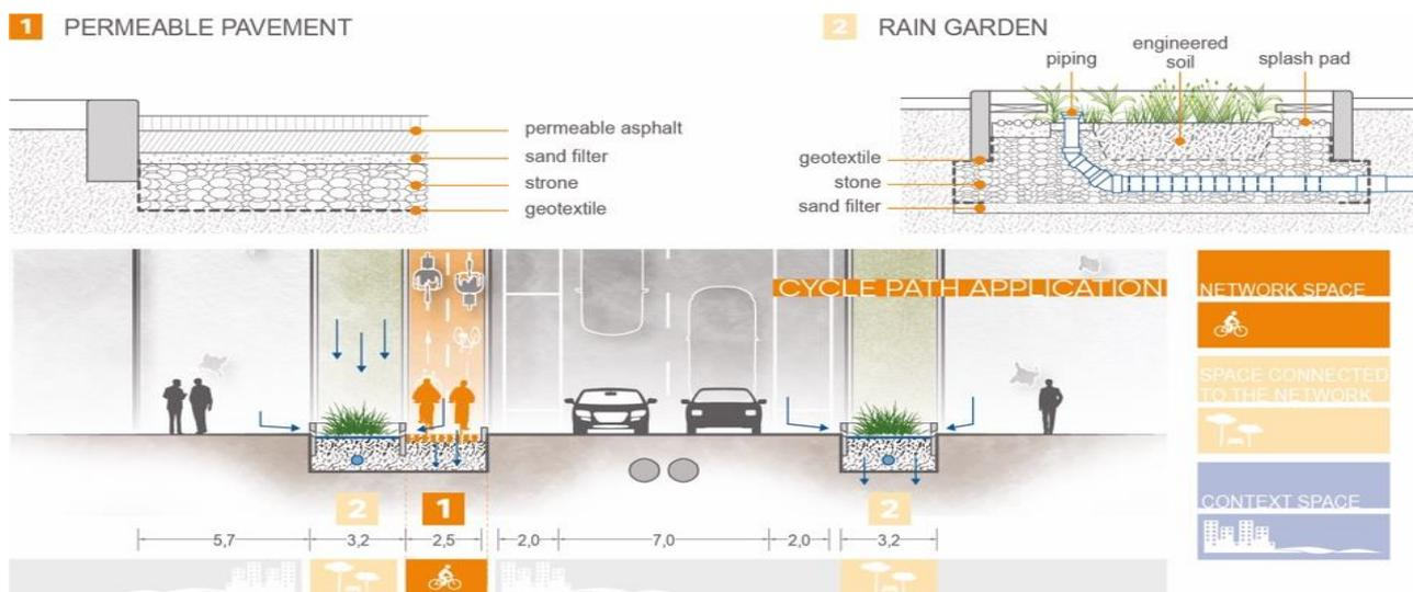
**Figure 12:** Philadelphia, section and planimetry of Permeable Pavement and Rain Garden: a hypothesis of application to the cycle path. Original drawing by arch. Angelica Nanni.
