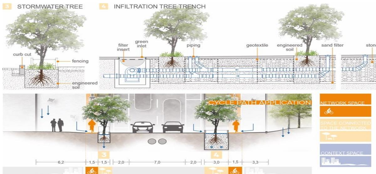
**Figure 13:** Philadelphia, section and planimetry of Stormwater Tree and Infiltration Tree Trench: a hypothesis of application to the cycle path. *Original drawing by arch. Angelica Nanni.*
