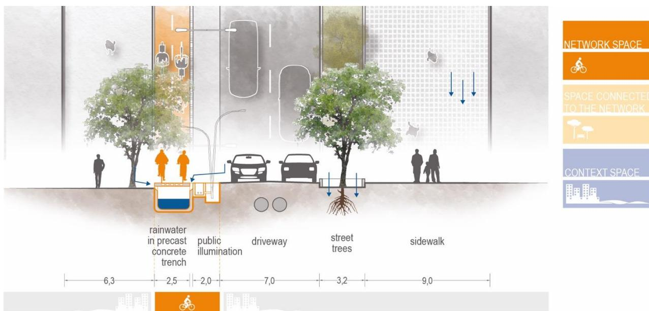
**Figure 9:** *The Copenhagenize Current* the design project for a prefabricated canal below the cycle path by Mikael Colville Andersen and Steve Montebello. *Original drawing by arch. Angelica Nanni.*
