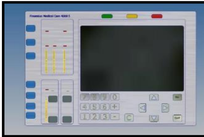
Figure 8: Hemodialysis machine display section designed using Blender 3D that is assembled and each button could be programmed individually.
