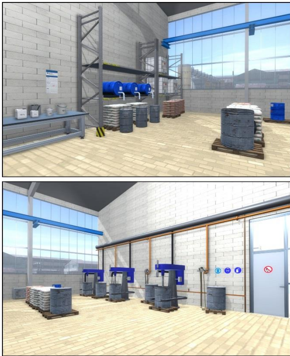
Figure 6: Virtual installation of the paint and coatings industry. On display in the upper screenshot of Fig. 6, there are dispensers of chemicals. The lower screenshot shows a workplace that is equipped with basket mills.
